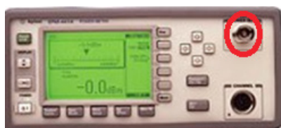
Figure 1. 50 MHz 1 mW Reference.
