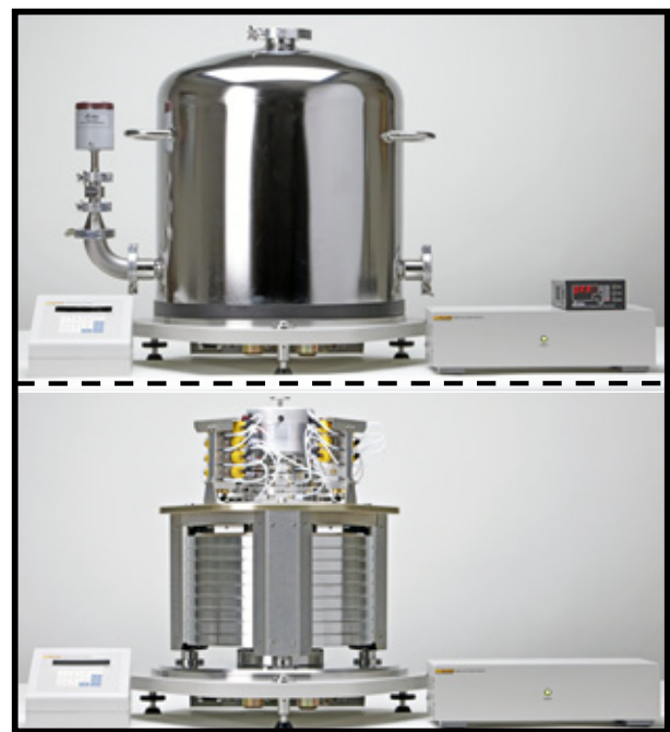
Figure 4. Picture of PG9607 complete (above) and with vacuum bell jar removed (below).
