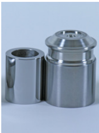
Figure 2. Picture of the 20 cm 2 area piston-cylinder.
