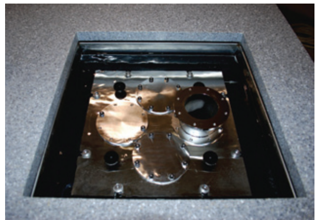
Figure 6. Chamber Submersed in Fluid Bath.
