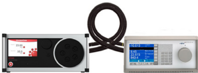
Figure 4. Chilled mirror connected to RH test chamber with sampling tubes.
