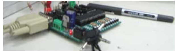
Figure 6. Manufactured circuit of the new fabricated decade resistance.
