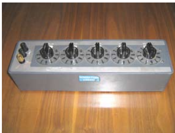
Figure 1a. Resistance box with five decades.
