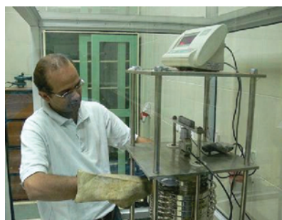
Figure 1. Using 1kN DWM to calibrate a load cell.
