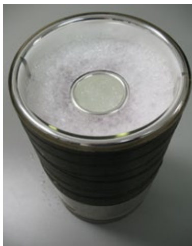
Figure 2. Fully prepared ice bath. Smaller dewar flask (center) is placed in a secondary bath in larger outer dewar flask to provide maximum thermal isolation and stability.
