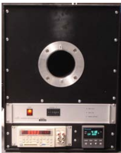
Figure 4. A blackbody cavity, with a length of 200 mm and maximum aperture diameter of 120 mm, enclosed in a uniform-temperature furnace. The effective emissivity is at least \epsilon_{bb} = 0.991 .
