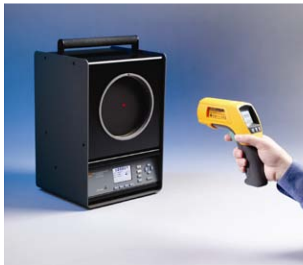
Figure 6. A flat-plate calibrator, with a diameter of 150 mm and emissivity of 0.95, being viewed by an infrared thermometer. Photo courtesy of Fluke Corporation, Hart Scientific Division, reproduced with permission.
