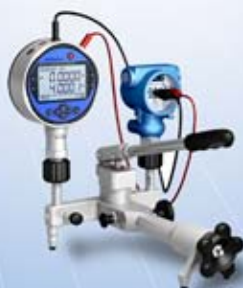
Pressure Calibration in the Field
