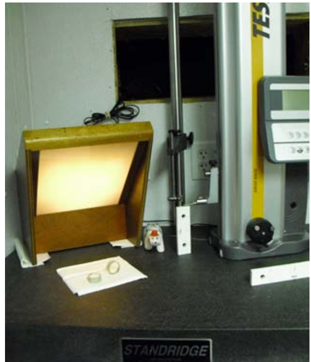
A monochromatic light with two optical flats in the mobile calibration unit.
