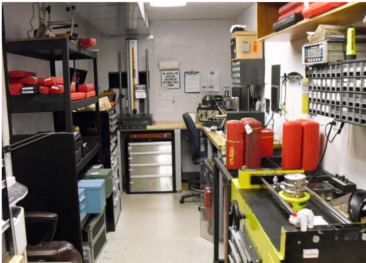
AMCS's mobile calibration lab is their newest unit: a 45 foot long enclosed container trailer, equipped with standards for maintaining precision and construction tools for about 25 different clients in the oil industry.
