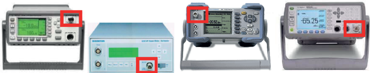
Figure 1. 1 mW (0 dBm) 50 MHz power reference calibrator on power meters.
