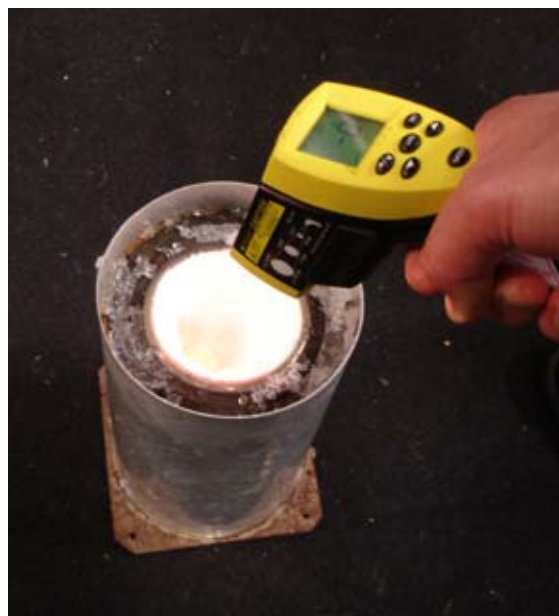
Figure 7. Measurement of an ice-point blackbody. The blackbody is a cavity carved into shaved melting ice inside a Dewar. While the ice is melting, its temperature is naturally maintained at a temperature of 0°C, so a separate reference thermometer is not required (see Ref. [1] for more details concerning the ice point).
