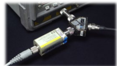
Figure 9. An example of a power splitter employed for precision levelling in a spectrum analyzer calibration application where the device shape and labelling help to easily identify its port configuration.
