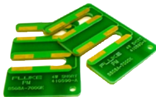
Figure 1. Small shorting devices are shown here. Specially made circuit boards, supplied with Fluke's 8508A DMM, provide both ohmic and thermal zeros for quick stabilization.
