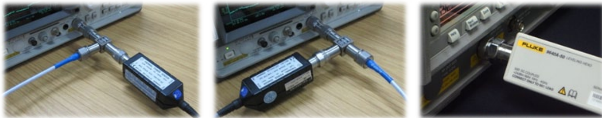
Figure 10. A power splitter correctly configured (left) and incorrectly configured (center) for precision leveling. On the right, a direct connection from the leveling head of an RF Reference Source.
