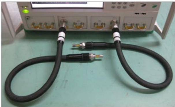
Figure 3. Phase and level stable cables used for Vector Network Analyzer (VNA) test port connections. VNA test port cables are extremely flexible, maintaining loss/phase characteristics when moved and flexed (extremely expensive).
