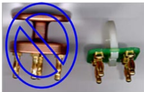
Figure 1. Small shorting devices are shown here. Specially made circuit boards, supplied with Fluke's 8508A DMM, provide both ohmic and thermal zeros for quick stabilization.
