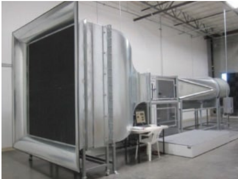
Figure 1. Photos of Aero-Subsonic Wind Tunnel (AWST1) and wind sensor under test (on the right).
