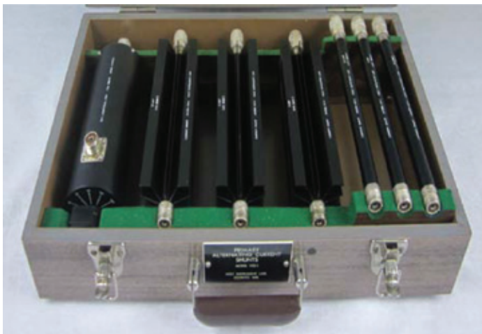
Figure 2. Shunt types used: Holt (model HCS-1) and Fluke (model A40/A40A).
