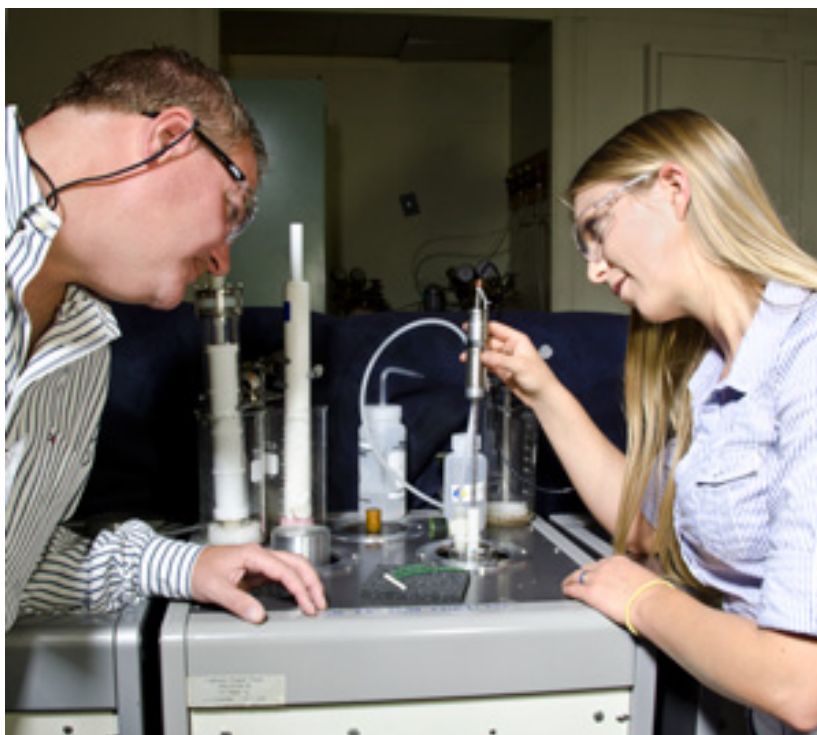
PML physicist Michal Chojnacky (right) demonstrates the method used to calibrate platinum resistance thermometers. At left is sensor designer Chris Albert.
