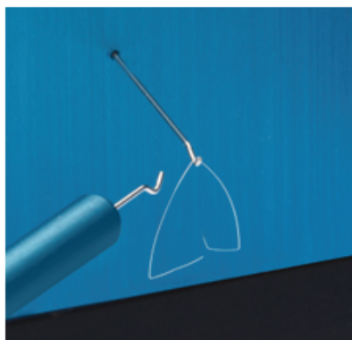
Figure 2. Aluminum handling tool with hook used for transfer of microgram weights.
