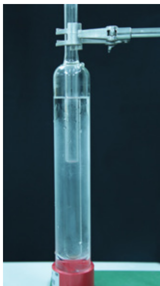
Cell water triple point, national measurement standard in Colombia.
