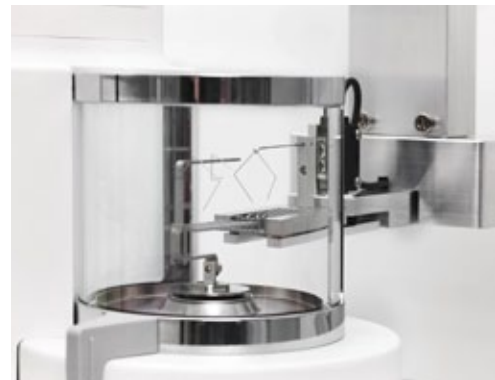
Figure 3. Robotic placement of wire weights on to the weighing pan using weight carriers with hooks.
