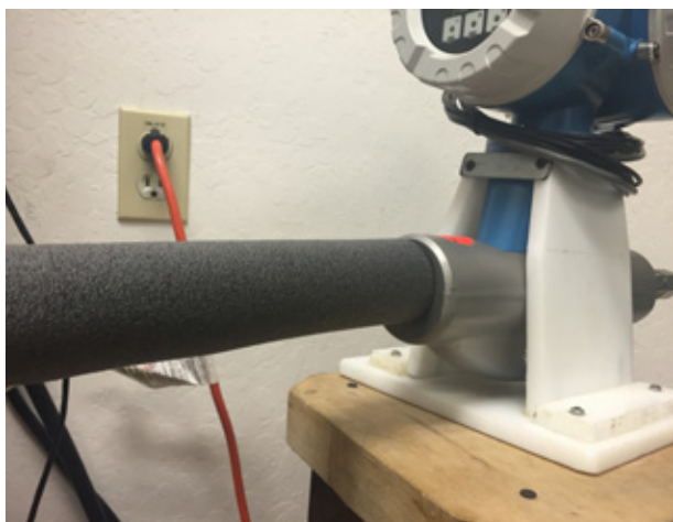
Figure 3. Calibration process with insulation and heat and cooling protection.
