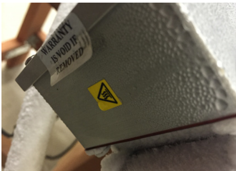
Figure 2. Calibration process without insulation, buildup of frost and freezing contacts.
