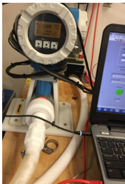
Figure 2. Calibration process without insulation, buildup of frost and freezing contacts.
