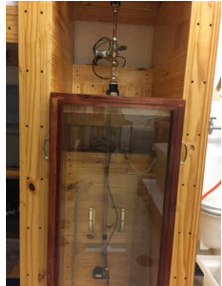
Figure 6. Low inertia turbine meter installed for flow stability assessments.
