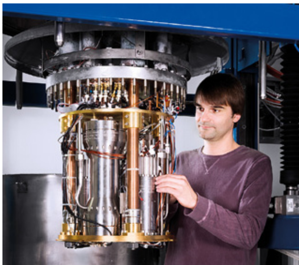
PTB scientist Christof Gaiser with the core of the dielectric-constant gas thermometer. The different silver-colored pressure vessels have special capacitors which are filled with helium to carry out the measurement that takes place inside them. Credit: PTB
