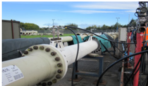
Figure 18. 14", 0.556β cone meter with verification system and verification system display.
