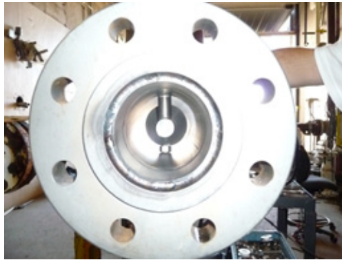
Figure 23. 4", 0.63 \beta cone meter with trapped nut and verification result.
