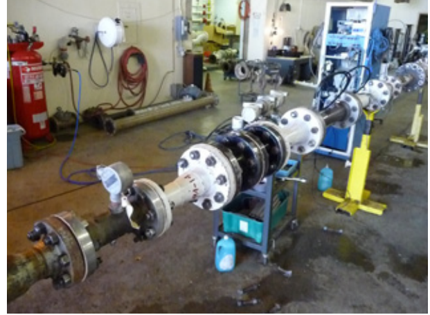
Figure 15. 3" Swirl Generator + Expansion 9D up.
