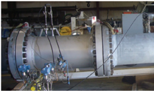
Figure 21. 26", 0.669 \beta cone meter at CEESI with verification system and verification system display.
