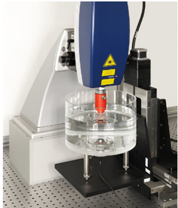
Measurement setup during a measurement with the vibrometer. The vibrometer is located in the blue housing. The foil is placed in the red lens tube and lies on the water surface. Credit: PTB
