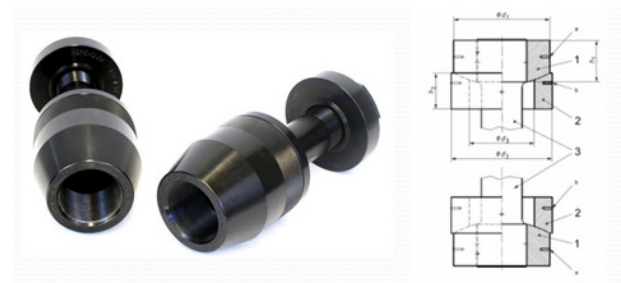
Figure 4. Tension Members with two ball nuts and two ball cups. Tensile force transducers should be fitted with two ball nuts and two ball cups
