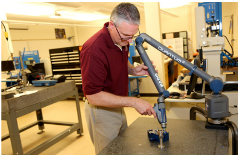
Kevin Ruediger, a Butler County Community College associate professor and coordinator of BC3's metrology program, demonstrates measuring the interior of a geowidget with a tactile probe attached to the program's new state-of-the-art $90,000 FARO Quantum S measurement tool in BC3's metrology lab on June 6, 2019. The Quantum S will allow his students to measure in three dimensions simultaneously. "Students ... are going to be blown away by it," he said. "This is just beyond anything else we have."
