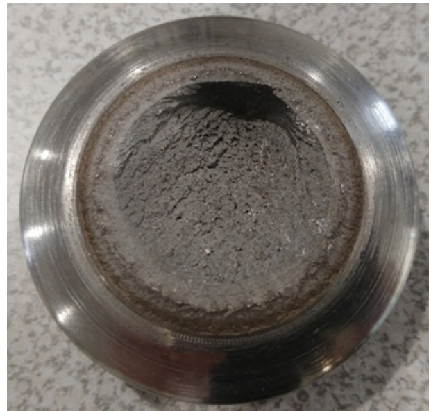
Figure 2. Grade 8 Bolt that failed at 120,000 lbf and close to 350,000 load cycles
