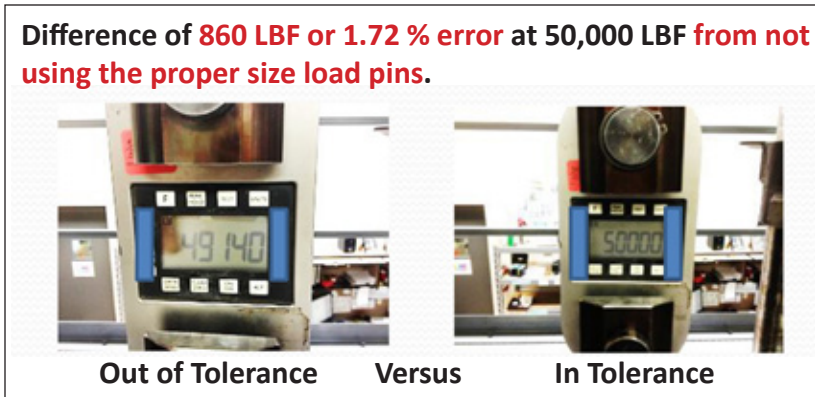
Figure 9. Tension Link Difference in output with pin size
