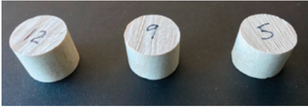
Figure 5. Small, numbered cylinders used to make and compare measurements with dial indicators and analog and digital micrometers.
