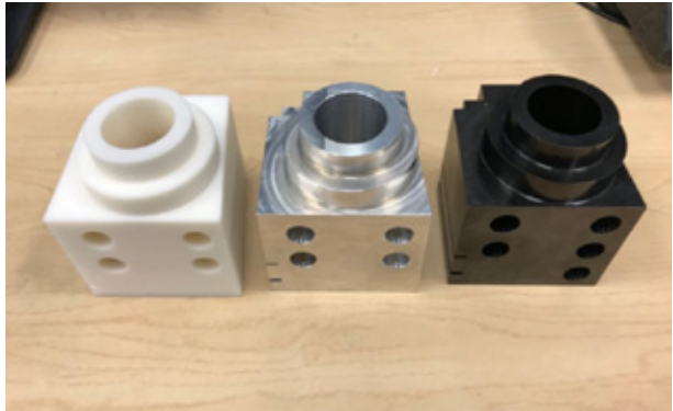
Figure 7. CMM artifact manufactured with 3 different materials employed for the dimensional measurement competency testing.
