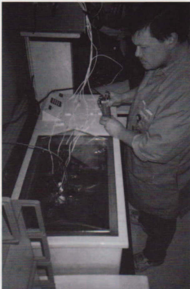
Figure 3. Dan Rumbold, Senior Metrology Technician at Verizon, utilizes a high quality temperature bath for the measurement of standard resistors
