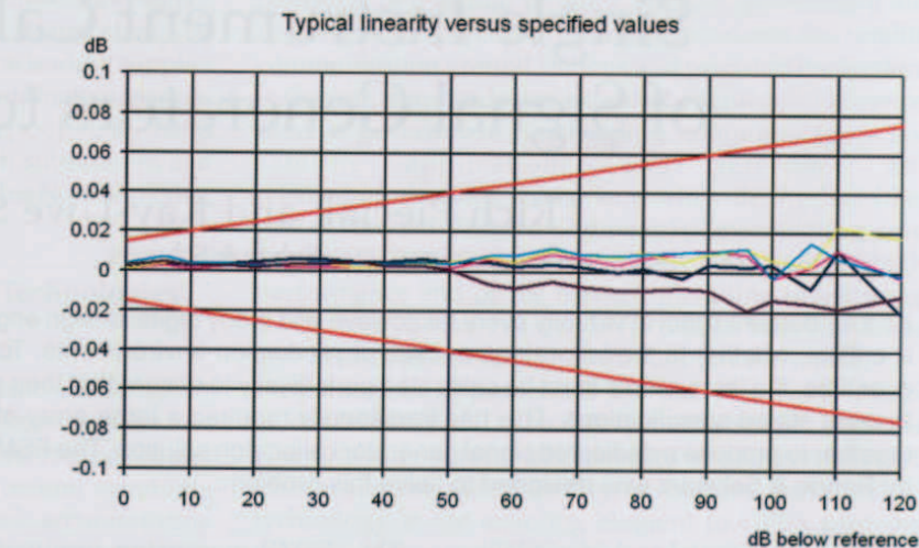
Figure 2. The actual linearity performance of the FSMR receivers is well within the specified limits.
