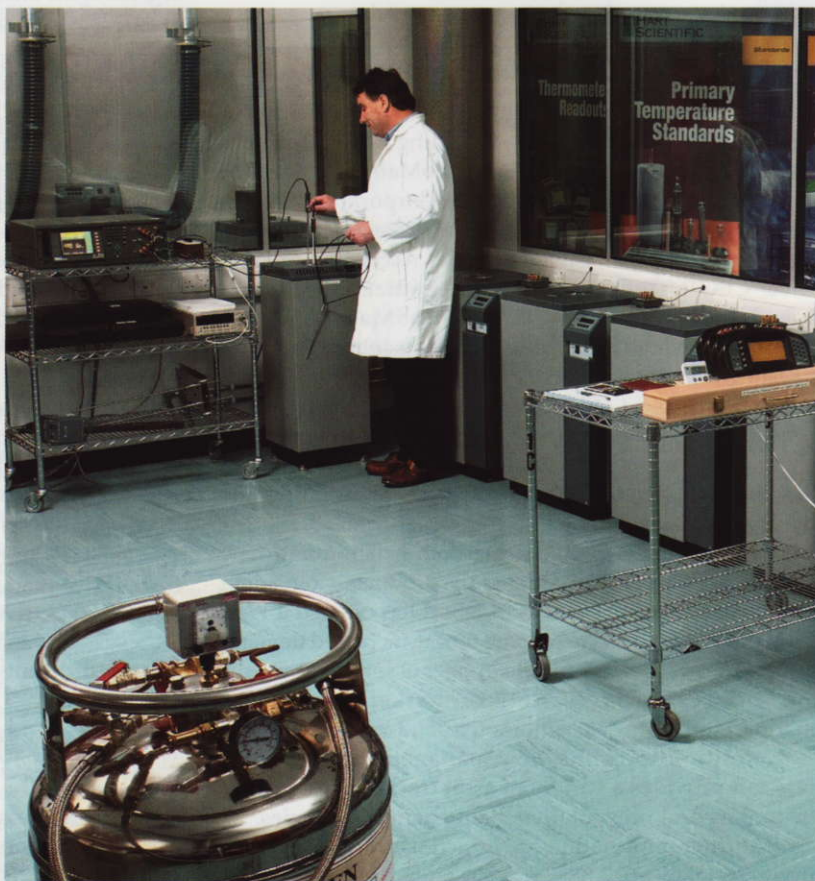
Lab manager Peter Crisp removes an SPRT from a Hart 9117 Annealing Furnace.
