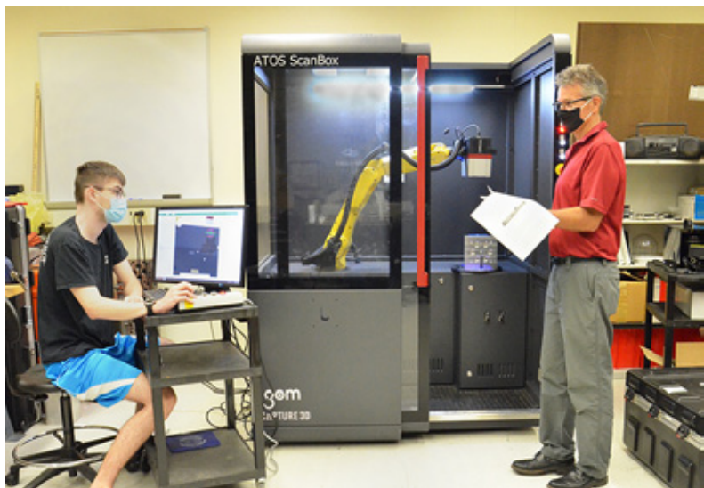
Undergraduate Research Assistant Ryan Gorman, left and Dr. Ed Morse working with a new ATOS ScanBox optical measuring machine. Credit: Photo courtesy of UNC Charlotte
