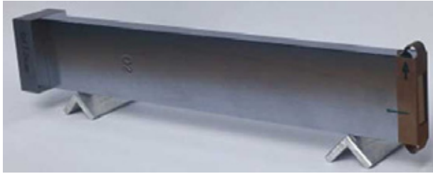
Gauge block made of single-crystal silicon. Dimensions: 197 mm × 35 mm × 9 mm. Credit: PTB
