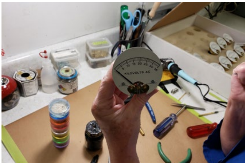
Q.C. testing of a product run of Hoyt panel meters.
