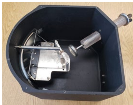
A Sensitive Research Model ESH with high and low ranges selected and meter movement detail.
