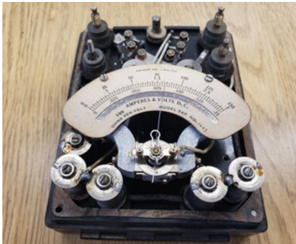
A Weston Model 540 DC Volt-Ammeter, circa 1895.
