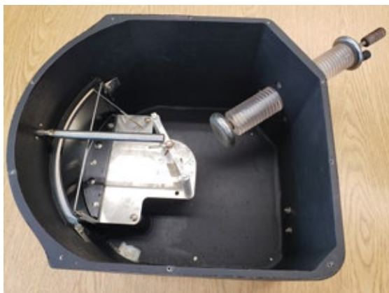
A Sensitive Research Model ESH with high and low ranges selected and meter movement detail.
