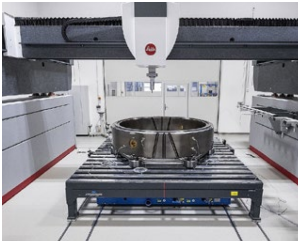
Measurement of the gear measurement standard on PTB's large CMM. Credit: PTB
